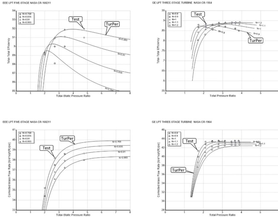
Figure 3: Calculated and measured turbine maps
