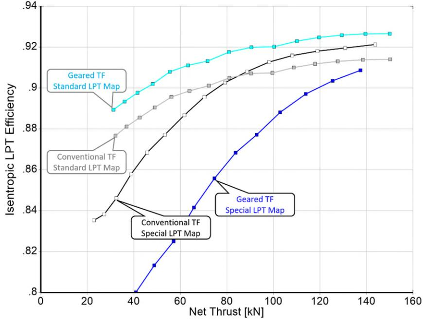
Figure 7: LPT efficiency along the SLS ISA+15K operating line
