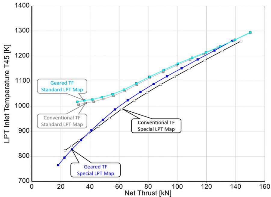
Figure 12: LPT inlet temperature for the SLS ISA+15K operating line
