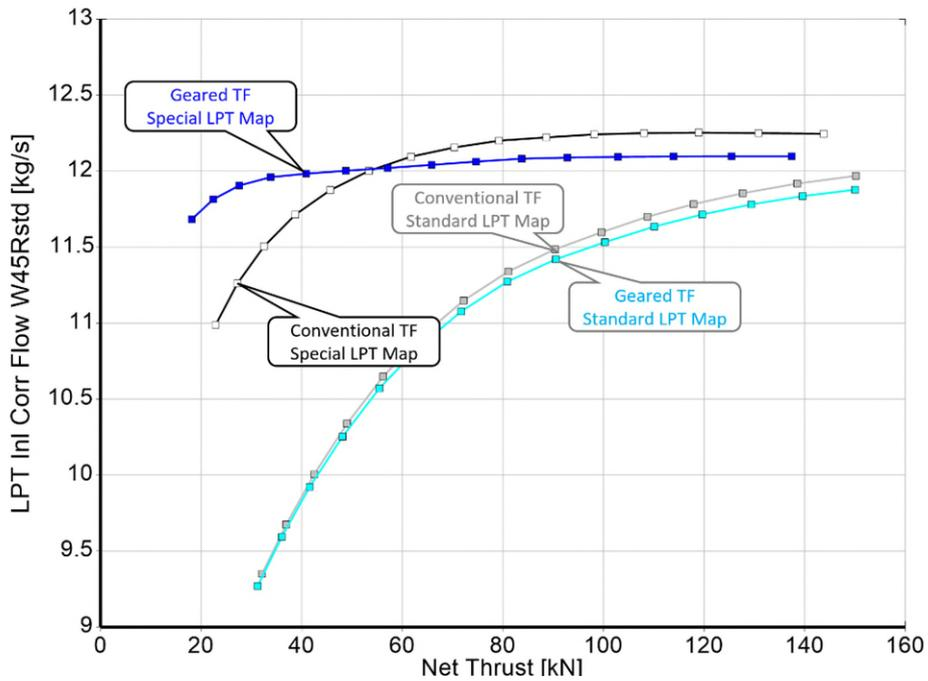
Figure 8: LPT corrected flow along the SLS ISA+15K operating line
