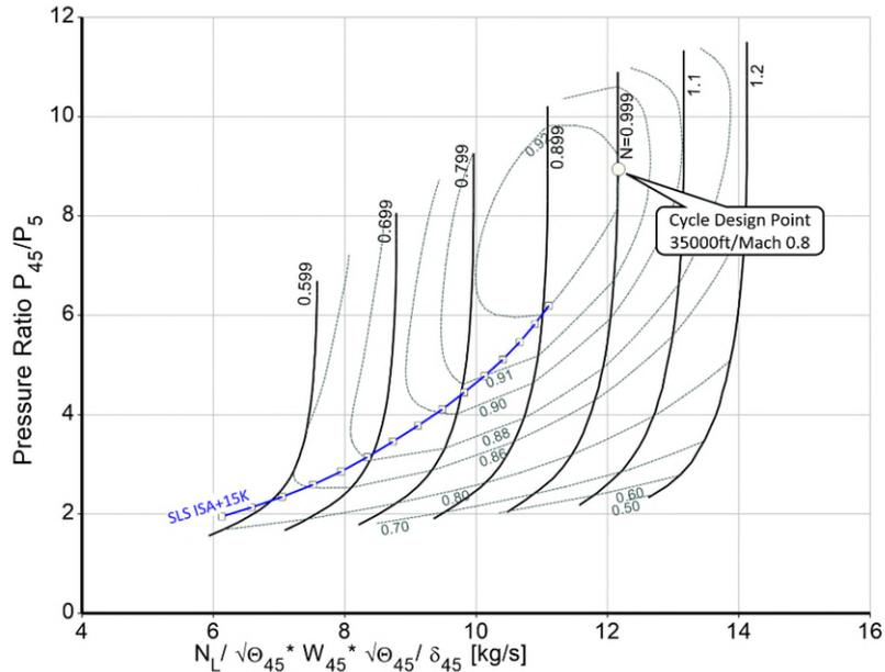
Figure 5: Operating line in the LPT map, conventional turbofan
