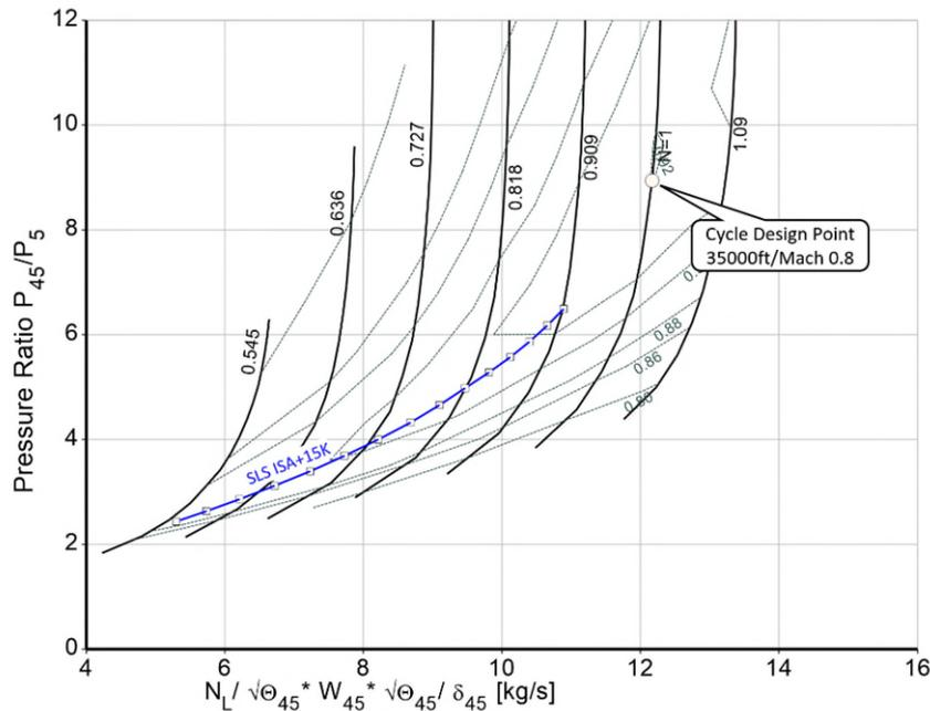
Figure 4: LPT Operating line in the scaled GasTurb Standard map
