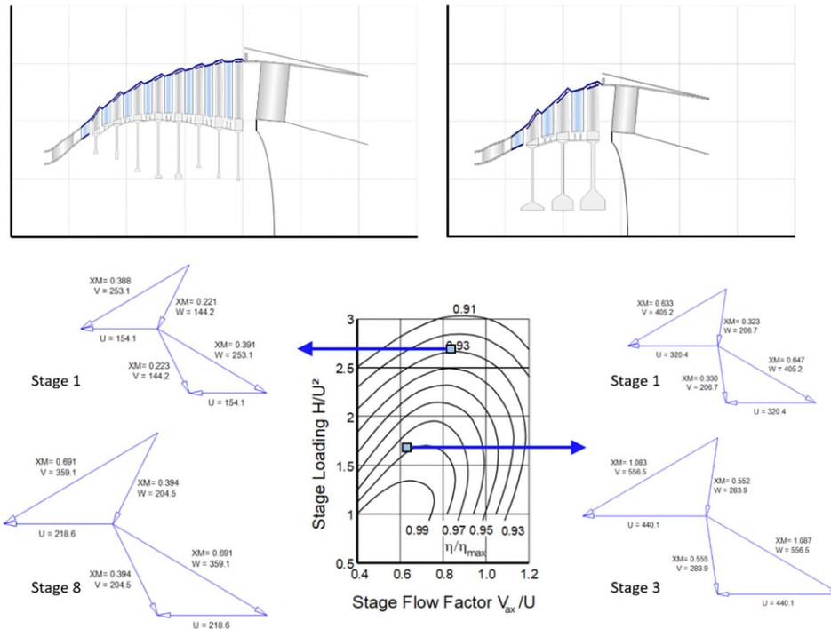
Figure 2: Flow-paths and velocity diagrams of the LP Turbines
