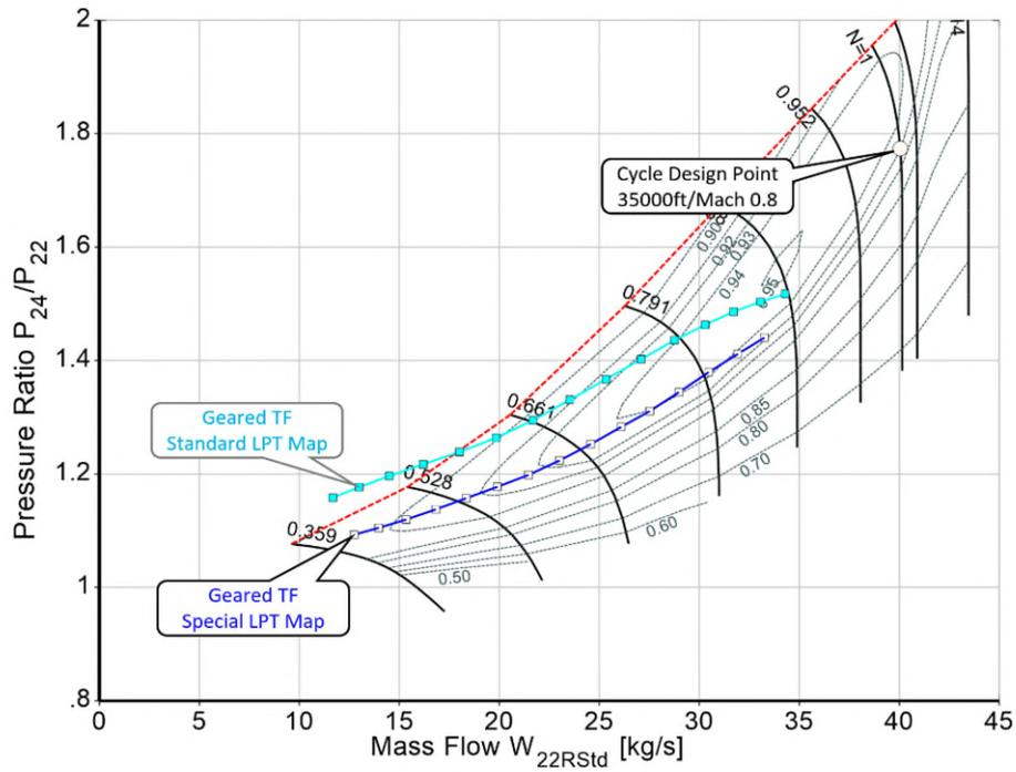
Figure 9: Booster operating lines for the geared turbofan
