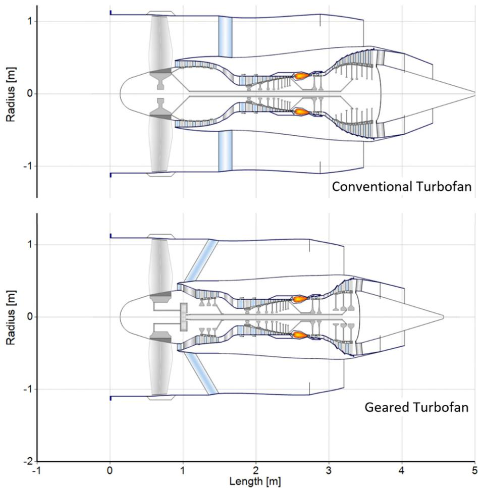
Figure 1 Conceptual design results for a conventional and a geared turbofan with common core and bypass ratio 12
