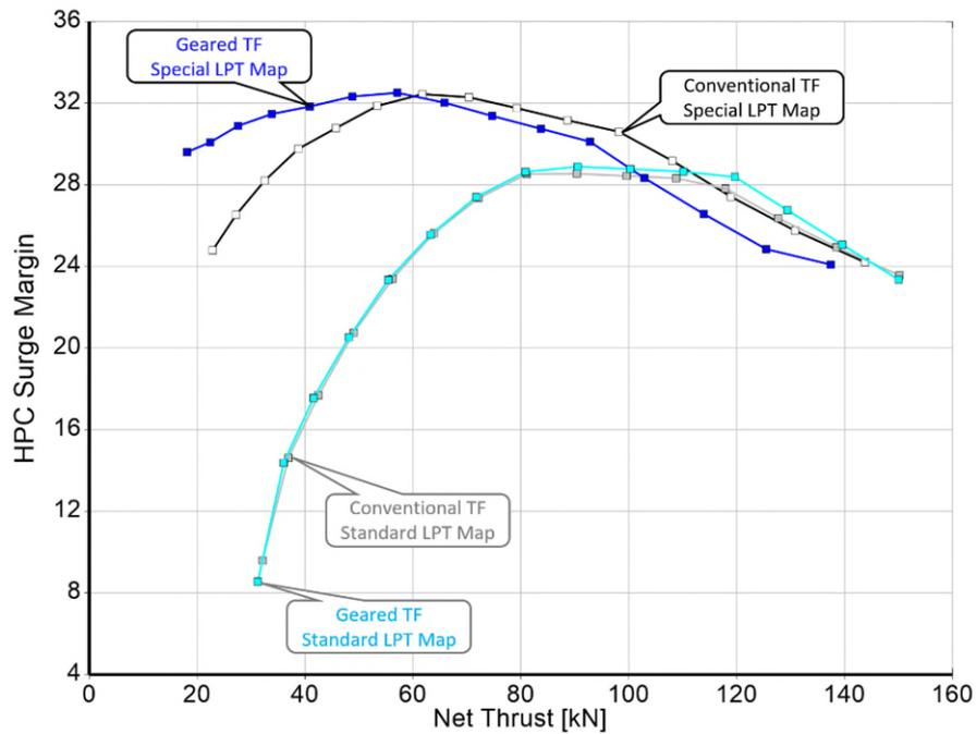
Figure 11: HPC surge margin along the SLS ISA+15K operating line
