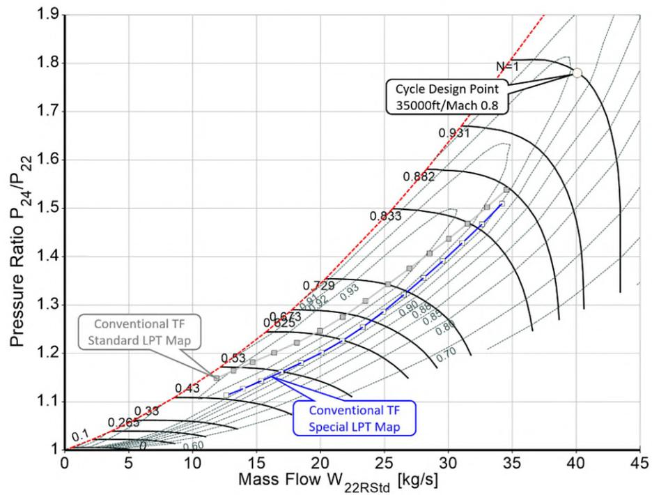
Figure 10: Booster operating lines for the conventional turbofan
